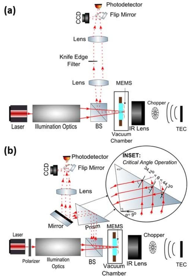
Fig. 3. Experimental setup for the characterization of single sensor element using different AC coupled optical readout methods: (a) Knife-edge method, KEM. (b) Critical angle method, CAM. The CCD was used to check the alignment of laser with the selected sensor for single MEMS pixel operation.
