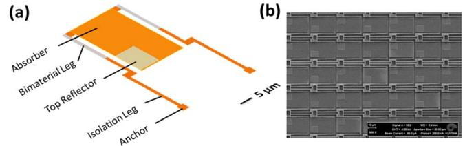
Fig. 1. (a) The geometry of single sensor element. (b) Scanning Electron Microscope (SEM) Image of a part of the array.
