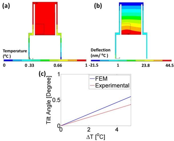
Fig. 2. FEM Analysis: (a) Thermal Gradient of the single sensor element due 1 °C input on the absorber where anchors are fixed at 0 °C. (b) Mechanical deflection analysis for the thermal gradient in (a). (c) Comparison of the tilt angles w.r.t. temperature using the experimental data and the FEM results.
