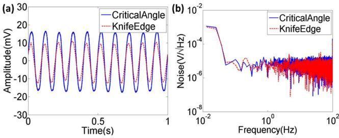
Fig. 5. (a) AC coupled photodetector signal obtained using a chopper blade (at 25°C) rotating at 10 Hz placed in front of an IR target (at 50°C) for knife-edge method (KEM) and Critical angle method (CAM). (b) Noise levels of the optical readout system for both methods.
