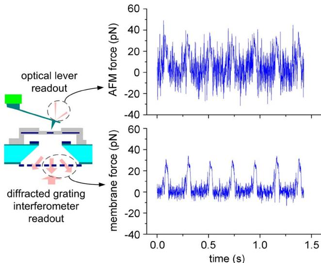
Fig. 9. Comparison of force curves obtained by the AFM cantilever and the membrane probe when a 2.8-N/m cantilever with quality factor of 3.8 was actuated against an 8-N/m membrane in fluid. The peak force on the cantilever was set such that SNR = 1.
