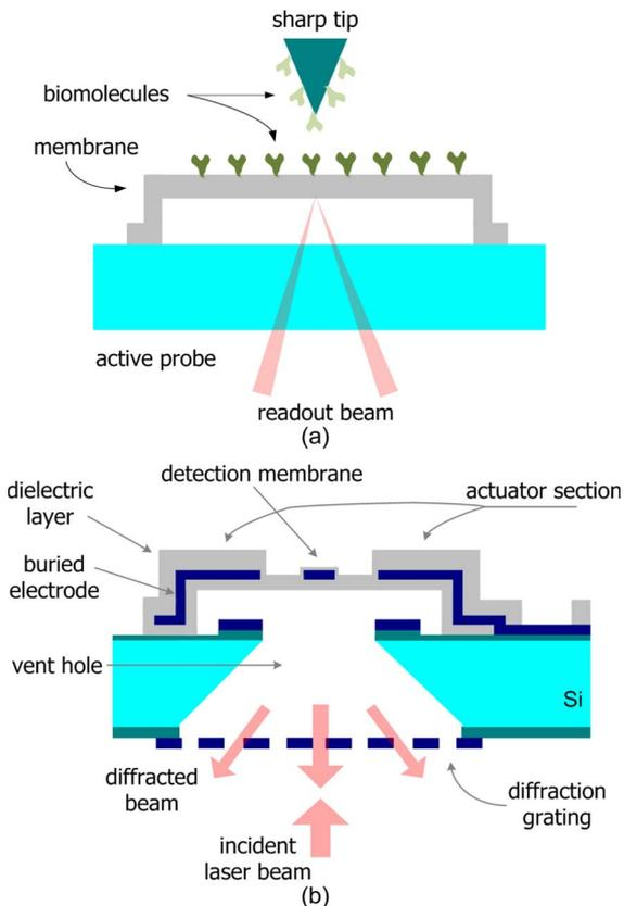
Fig. 1. (a) Generic schematic of a single-molecule experiment employing a functionalized active probe that is coupled with a functionalized sharp tip. (b) Schematic cross section of probe structure highlighting its different sections.
