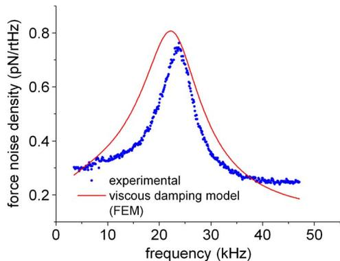
Fig. 8. Force noise spectrum of a 500- $\mu\text{m}$ -diameter force probe with 300- $\mu\text{m}$ -diameter detection membrane in fluid.
