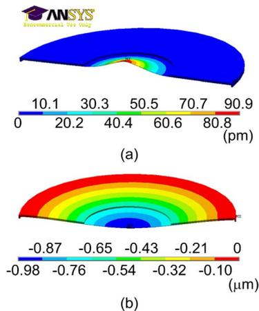
Fig. 2. FEM simulation of displacement profile of (a) the unbiased membrane when 100-pN point force is applied at the center and of (b) the membrane with applied voltage to the side electrodes to displace the center by 1  $\mu\text{m}$ . One-half of the membrane is shown.
