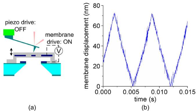
Fig. 7. (a) Actuation of an AFM cantilever by using electrostatic actuator of membrane probe. (b) Cantilever readout signal in fluid when the membrane was actuated by a ramp signal.
