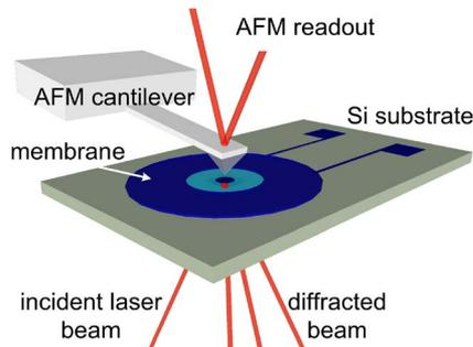
Fig. 4. Schematic of membrane probe coupled with AFM cantilever in the experimental setup.
