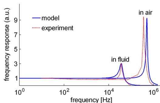
Fig. 6. Frequency response of a 200- $\mu\text{m}$ -diameter membrane in air and fluid.
