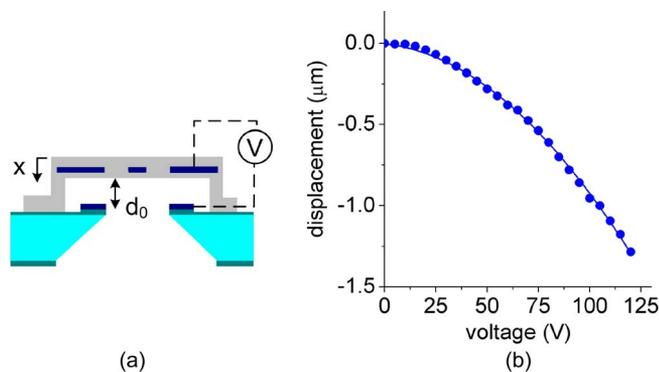
Fig. 5. (a) Schematic of integrated electrostatic actuator with side electrodes. (b) Displacement of a 200- $\mu\text{m}$ -diameter membrane with applied bias voltage.
