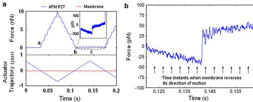
**Fig. 4** **a** Force (*top*) and displacement (*bottom*) trajectories of PZT and membrane actuators. A visible hydrodynamic drag (as signified by a kink in the force-time trace; see *inset*) manifests during PZT actuation, while membrane actuation at comparable speed does not
