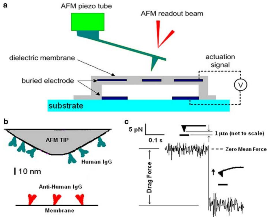
**Fig. 1** **a** AFM experimental setup: The experimental unit consists of an (electrostatic) actuation-capable membrane underneath a commercial AFM setup, with the cantilever deflection being monitored continually by conventional laser beam-bounce technique. **b** Functionalization of AFM tip and membrane: In the biomolecular pulling experiments, the cantilever tips were incubated with human IgG, and the membranes were incubated with anti-human IgG (see *Materials and methods*);
